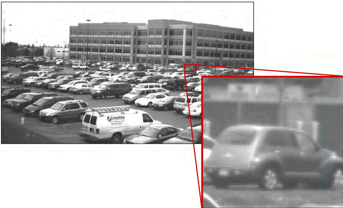
Single frame of digital video taken with UAV-Cam V2M using 30 degree FOV lens
